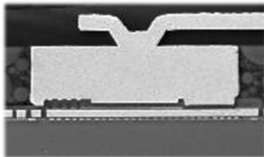
Direct Connect Cu Stud Low contact resistance, multi-via capture
